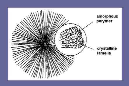
schemantic diamantic of spherulite
