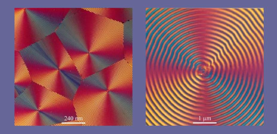
Micrograpy of spherulites in Polyhydroxybutyrate (PHB)
