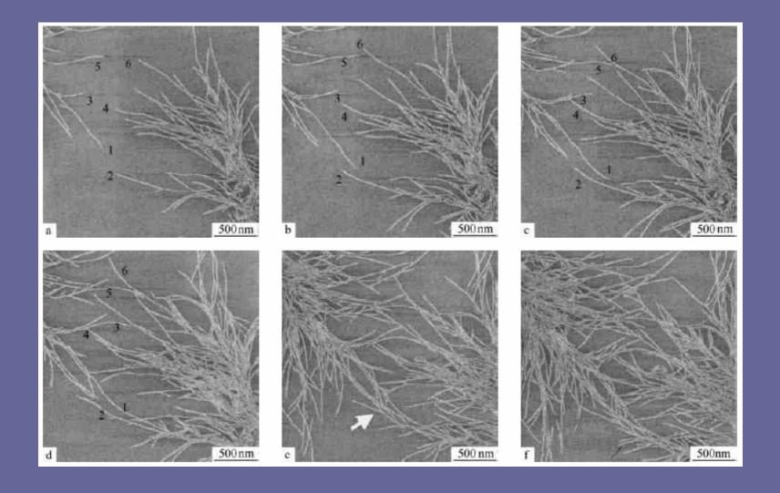
AFM phase images showing the growth of lamellae at the interface between two spherulites in a consecutive time sequence. The time interval between two images is about 6 min.
