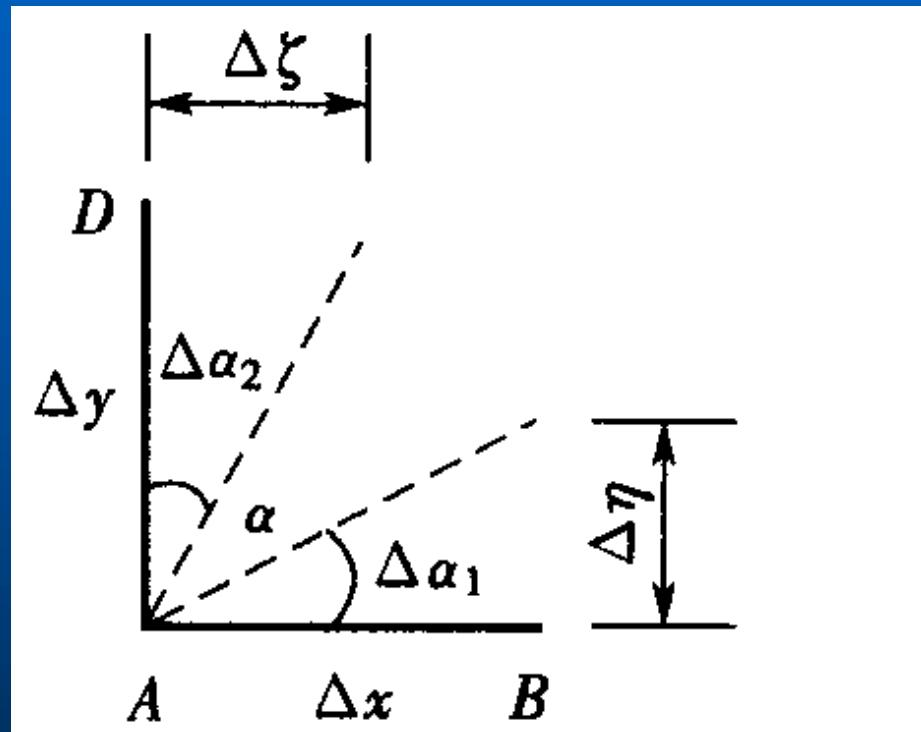
$$e_{xy} = e_{yx} = \frac{1}{2} \frac{\delta\alpha + \delta\beta}{dt} = \frac{1}{2} \left( \frac{\partial u_x}{\partial y} + \frac{\partial u_y}{\partial x} \right), \quad e_{yz} = e_{zy} = \frac{1}{2} \left( \frac{\partial u_z}{\partial y} + \frac{\partial u_y}{\partial z} \right), \quad e_{xz} = e_{zx} = \frac{1}{2} \left( \frac{\partial u_x}{\partial z} + \frac{\partial u_z}{\partial x} \right)$$
