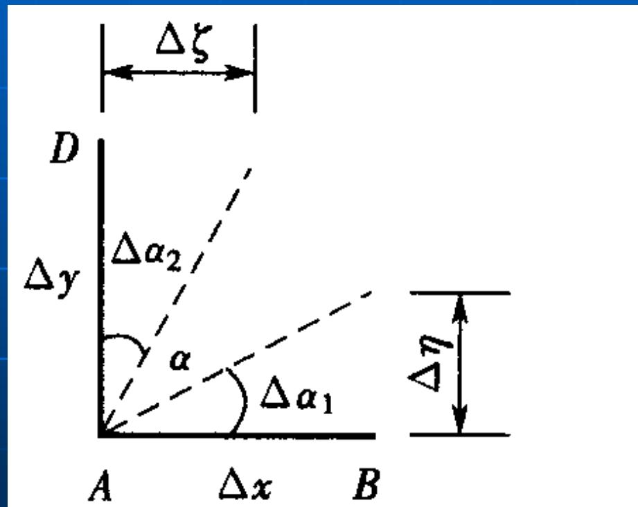
$$\omega_z = \frac{1}{2} \frac{\delta\beta - \delta\alpha}{dt} = \frac{1}{2} \left( \frac{\partial u_y}{\partial x} - \frac{\partial u_x}{\partial y} \right), \quad \omega_x = \frac{1}{2} \left( \frac{\partial u_z}{\partial y} - \frac{\partial u_y}{\partial z} \right), \quad \omega_y = \frac{1}{2} \left( \frac{\partial u_x}{\partial z} - \frac{\partial u_z}{\partial x} \right)$$
